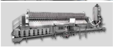
is a fully automatic weighing system for powder ingredients, granting constant quality and thorough control over technical rubber preparations.
