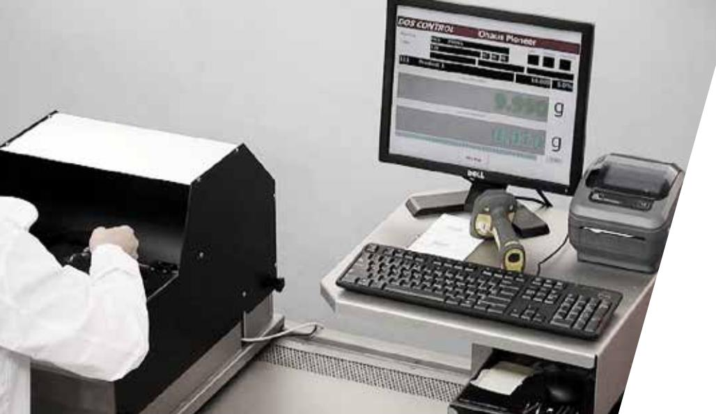
The check weight system facilitates recipe management, assisting the operator during the weighing process to control with precision every component of the recipe in order to guarantee the traceability of the operation with subsequent recipe and inventory control.
